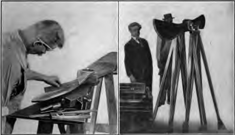
FIG. 21.—Testing shape of blade.
